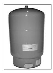
**Supply Storage Tank:** A supply storage tank must be used in a system with less than 50 gallons or 5 gallons per ton - whichever is greater - of liquid solution. The tank prevents rapid cycling of the compressors and acts as a reservoir for chilled liquid solution.
