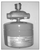
**Expansion Tank and Air Scoop:** The expansion tank and air scoop assembly is used to compensate for the expansion and contraction of liquid solution in the system. The air scoop eliminates air entrained in the liquid solution.
